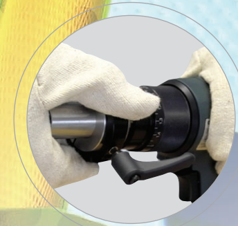
Feed unit twistable in cramped working areas
