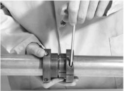
**Note** Make certain that the clamping shells are parallel, positioned closely to each other and locked in place.
