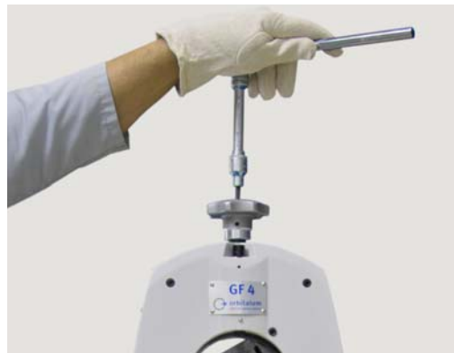
Adjusting the pipe dimensions using a ratchet with a number eight nut in the hand wheel
