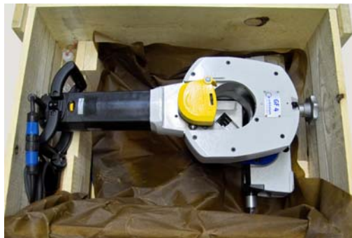
Position of the machine in the transportation case upon delivery.
