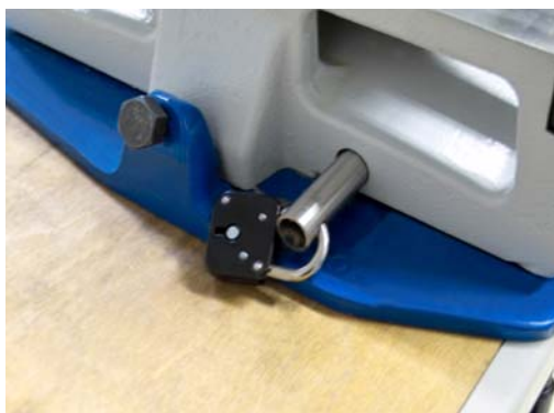
Locking mechanism of the slide housing prevents unauthorized usage and theft
