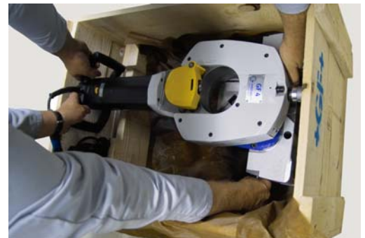
Transport and fit the machine with the aid of a second person or a crane or similar device.
