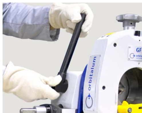
Adjusting the clamping jaws
