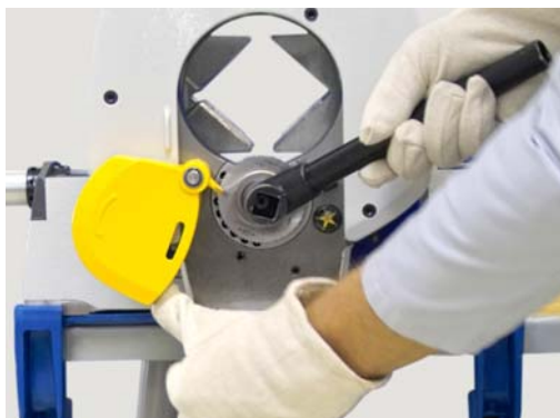
Tightening the saw blades and bevel cutters
