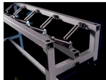
Pipe feeder for accurately feeding long and heavy pipes into GF and RA machines (page 18)
