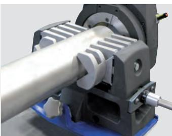
Clamping shells or jaws for deformation- or corrosion-free clamping of tubes (page 16)
