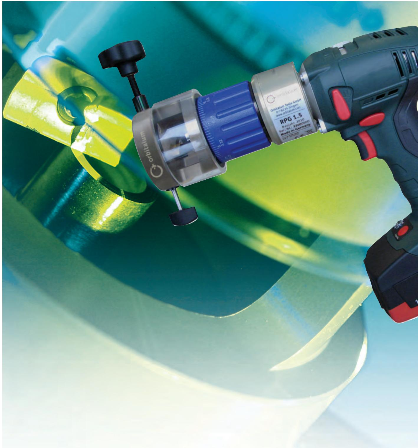
The required, high-quality tube end preparation for orbital welding.
