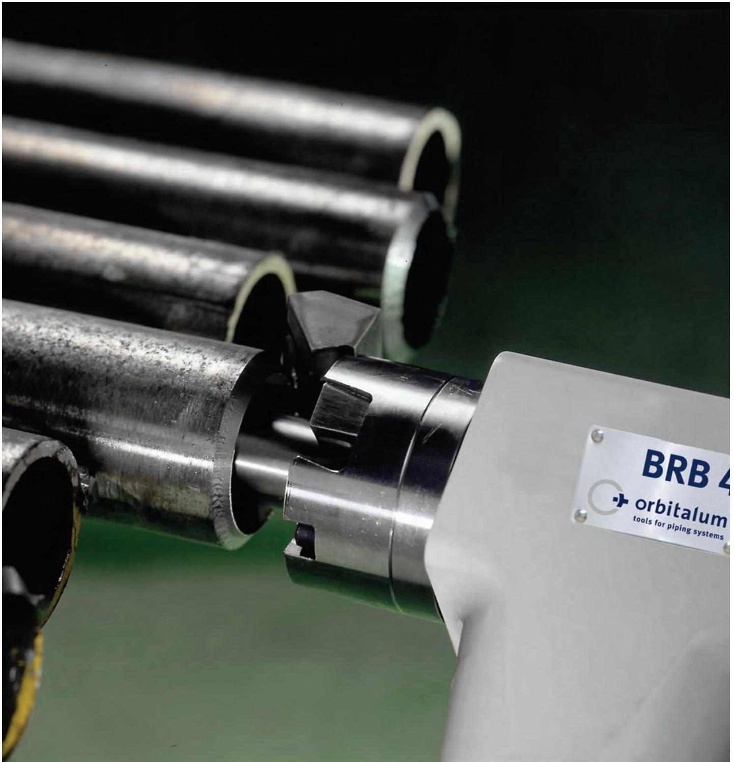
Powerful and robust boiler pipe preparation machine.
