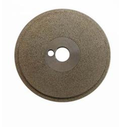
Exchangeable grinding wheel diamond-coated on both sides for optimal performance. For 1.0 and 1.6 mm (0.039 and 0.063 inch) electrodes we recommend the standard grinding wheel. For 2.0 mm (0.078 inch) and larger electrodes, a medium to coarse grained grinding wheel is advisable.
