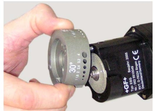
3. Slide a 2.4 mm pin through cross hole and motor shaft (rotation of the grinding wheel is prevented).
