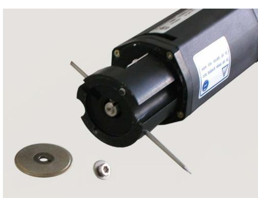
7. Tighten the Torx screw and assemble the ESG Plus grinding head to the motor.
