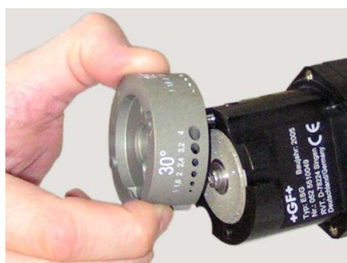
3. Slide a 2.4 mm pin through cross hole and motor shaft (rotation of the grinding wheel is prevented).
