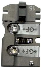
To cut tungsten electrodes to fixed length. For electrode diameters 1.0; 1.6 and 2.4 mm (0.040; 0.060 and 0.095 inch). Fixed cutting lengths: 12; 13; 15 and 17 mm selectable (0.470; 0.500; 0.600 and 0.670 inch). Other cutting lengths possible.
